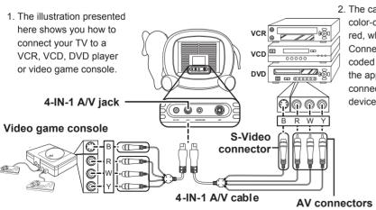
2. The cables are color-coded (black, red, white, and yellow). Connect each colorcoded cable to the appropriate connector on your
